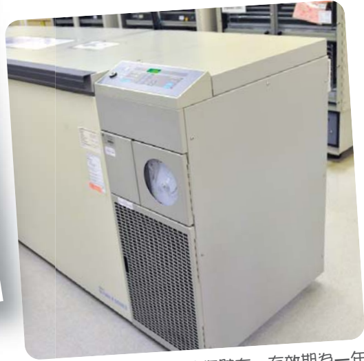
血漿放置在攝氏-70°C的冰櫃貯存，有效期為一年 Fresh Frozen Plasma products are stored in freezer at -70°C, the shelf life is 1 year.
