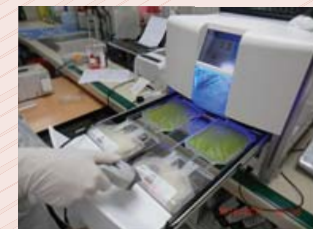
化驗部人員為血漿進行病原體滅活處理 A LAB staff performing pathogen reduction treatment of plasma units
